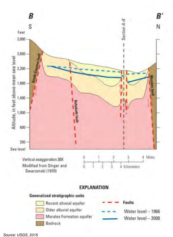
Figure 2-7: USGS Cross Section B-B'
