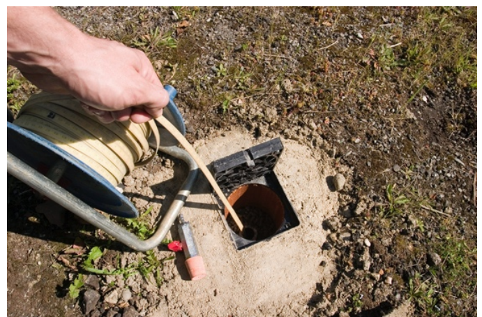
Measuring a dedicated monitoring well using an electronic sounder.
